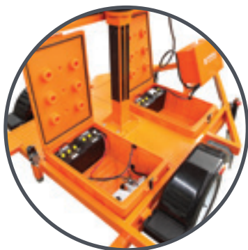
STANDARD MESSAGE SIGN BATTERY STORAGE.
